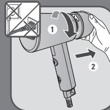
**EN** Remove the water tank by unscrewing it.
