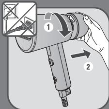
**EN** Remove the water tank by unscrewing it according to the marking.
