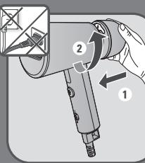
**EN** Return the water tank to its place by screwing it according to the marking until completely set. Make sure that water tank is fully set in place.
