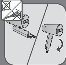
**EN** Always unfold the steam head until it is locked before any use of the appliance. Never steam when folded.
