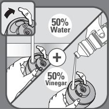
**EN** Fill the water tank with 50% water and 50% white vinegar.
