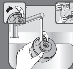
**EN** Rinse the water tank. Once rinsed, fill the water tank with 100% water. Close the water inlet cap.
