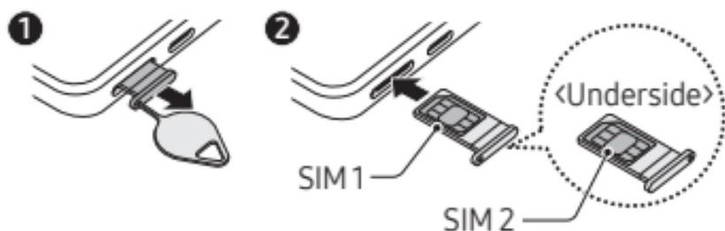
Insert the ejection pin into the tray's hole to remove the tray.
